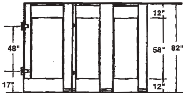
Headrail Braced (most commonly used)
