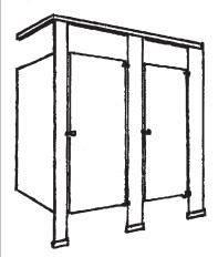
Available in four construction styles - headrail braced, ceiling hung, floor to ceiling and floor supported. Color to be selected from manufacturer's stand charts for this product.
