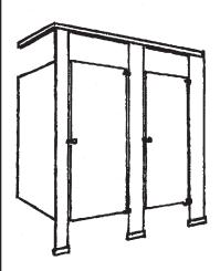
Available in four construction styles - headrail braced, ceiling hung, floor to ceiling and floor supported. Color to be selected from manufacturer's stand charts for this product.
